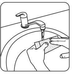
**Caution** ! Let the foam filter dry completely before placing it back into place.
